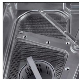
If the filter is missing or not inserted correctly, the SMARTRONIC displays a warning.
